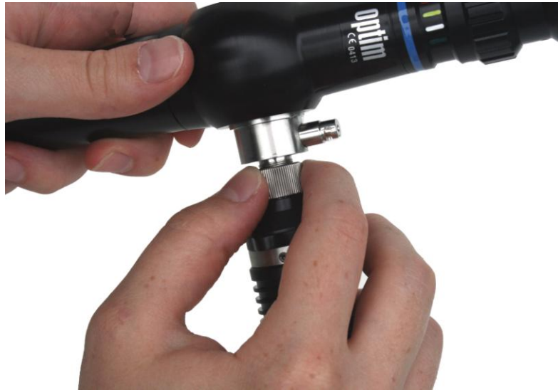
Figure 2. Attaching the Portable Light Source to a scope
