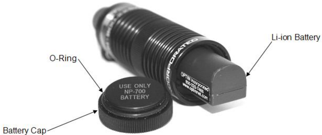
Figure 4. Removing the battery cap and inserting and removing the Li-Ion Battery
