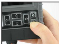
Step 3: Aim the camera at the selected target object. Press the CAMERA icon to take a JPG image or RECORD to record an AST video.
