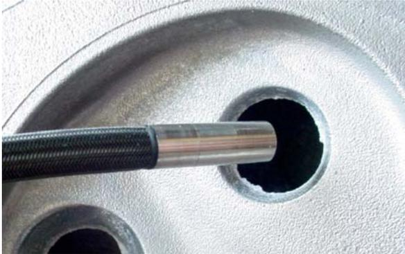
If a bend must be negotiated, articulate the tip in the direction of the bend to keep the tip from buckling. If the scope is obstructed by objects or bends, rotate the tube back and forth while moving it forward.
