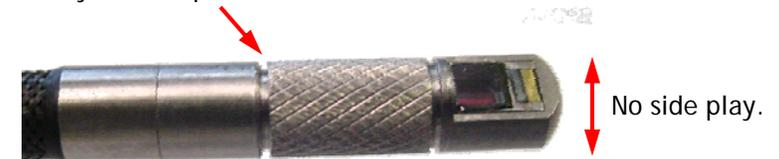
Always keep the Tip Cap or an adapter installed to protect the Tip threads.
