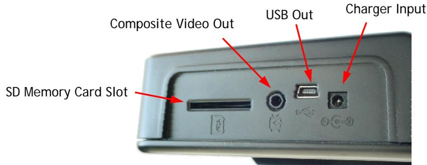
The video display shows live video and captured still or moving images. It can output live video to an external monitor via a composite signal connector and the included cable.
