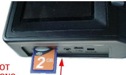
**Caution** - Do not remove the SD memory card during image capture operations, data will be lost and the memory card may be damaged.
