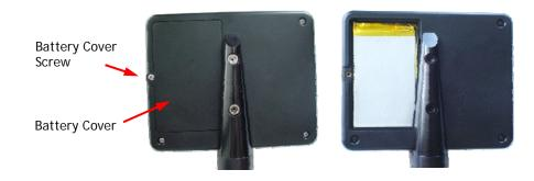
Carefully expose the battery wires and connector. Pull the connector apart and connect new battery. Replace the battery in its compartment and replace the cover and screw.
