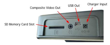
The video display shows live video and captured still or moving images. It can output live video to an external monitor via a composite signal connector and the included cable.
