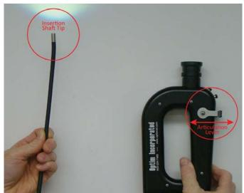
**Straight** – When inserting or removing the insertion shaft from inside an area the shaft tip must be in the straight position (no articulation); this is achieved when the articulation lever is in the straight position.
