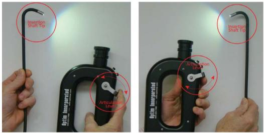
**Up/Down** – The insertion shaft tip can be articulated up/down, when the articulation lever is pushed forward or backward using your thumb.
